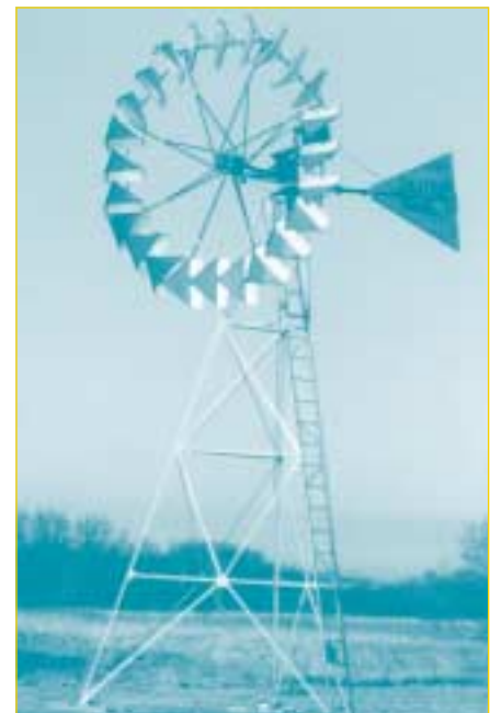
▲ Mechanical water pumping system.
